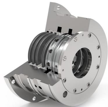
Carbon ring seals are usually made of graphite material and have self-allocating properties, which rely on the fluid resistance effect in the seal gap to achieve the seal effect.
